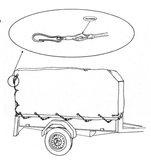
The long tarpaulin cord is fastened in front and on both sides the following way:
