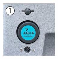
Fill the water tank by turning the lock (triangle) and pressing the lid in. The tank can hold approximately 65L.
