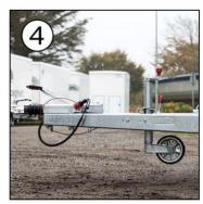
Wind the jockey wheel up and release the handbrake. If it is left for a long time, the brake shoes can get stuck.
