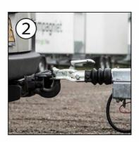
Reverse up to the trailer and place the coupling on the ball hitch. Press the handle down again and check it is seated correctly.
