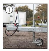
Put the handbrake on and turn the nose wheel down. Disconnect plug and safety wire. Then release the trailer.
