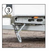
Wind down the support legs so that the trailer stays horizontal. The angle on the legs must be at least 45 degrees from the trailer.
