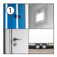
Close and <u>lock</u> cupboards, windows and doors. Secure any loose fittings and place heavy objects over the axel.
