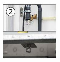
Locate the water intake in the technical compartment or on the side of the chassis under the trailer.
