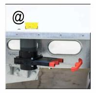
Pull the handle to empty the toilet tank. Flush with water to clean.
