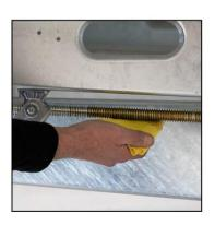
Locate the 4 treaded spindles for the support legs. Use a spray or cloth to apply lubrication.
