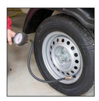
The wheel rims must be tightened with a pressure of 90 Nm (9 kilos). The cover must be pumped according to the tire description.
