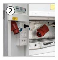
Locate the power inlet in the technical compartment or on the side of the chassis hangers under the trailer.
