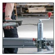
Locate the 3 grease nipples that are located on the inlet brake and the jockey wheel. Use a grease gun to fill.
