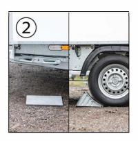
On soft ground, place plates under the support legs. On sloping ground, place wedges in front or behind the wheels.
