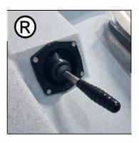
Pump with the handle next to the toilet to flush the toilet with water.
