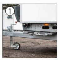
Prepare the trailer for driving (see disconnecting electricity, water and water). Wind the jockey wheel down and support legs (tight).
